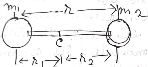
Figure A rigid diatomic molecule treated as two masses  $m_1$  and  $m_2$ , joined by a rigid bar of length  $r_0 = r_1 + r_2$
