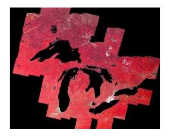
VARIATIONS IN ILLUMINATION AND VIEWING GEOMETRY BETWEEN IMAGES (FOR OPTICAL SENSORS) CAN BE CORRECTED BY MODELING THE GEOMETRIC RELATIONSHIP AND DISTANCE BETWEEN THE AREA OF THE EARTH'S SURFACE IMAGED, THE SUN, AND THE SENSOR. THIS IS OFTEN REQUIRED SO AS TO BE ABLE TO MORE READILY COMPARE IMAGES COLLECTED BY DIFFERENT SENSORS AT DIFFERENT DATES OR TIMES, OR TO MOSAIC MULTIPLE IMAGES FROM A SINGLE
