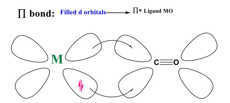
Back donation of electrons from filled d orbitals of metal to empty antibonding orbitals of CO
